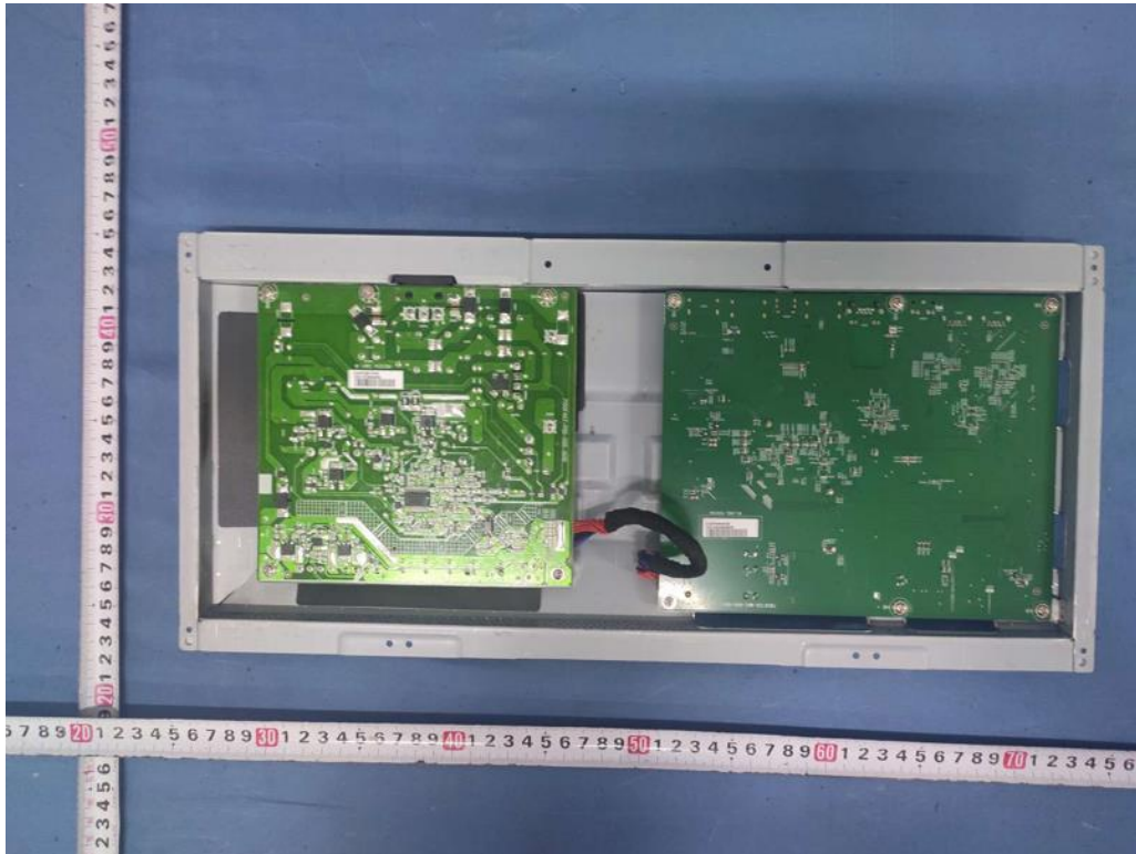
Figure 15. Internal view of EUT with power board 715GF467
