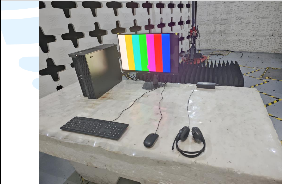
Radiated emission Test Setup (Above 1GHz)
