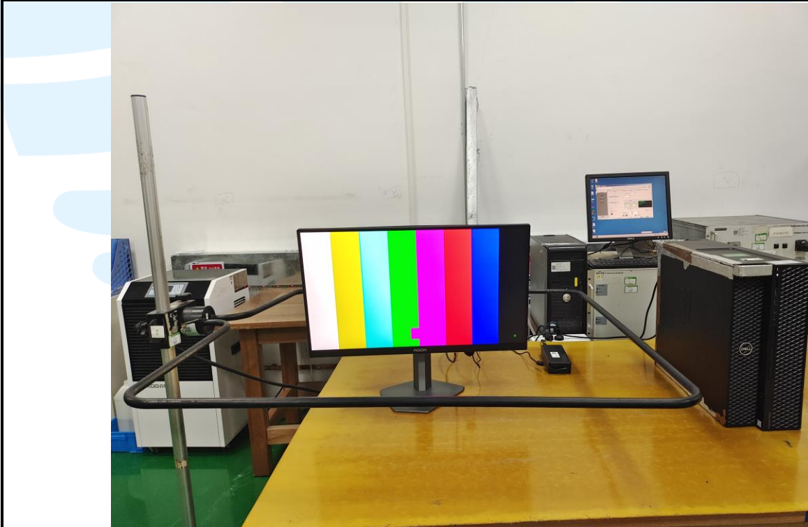
Power frequency magnetic field Test Setup
